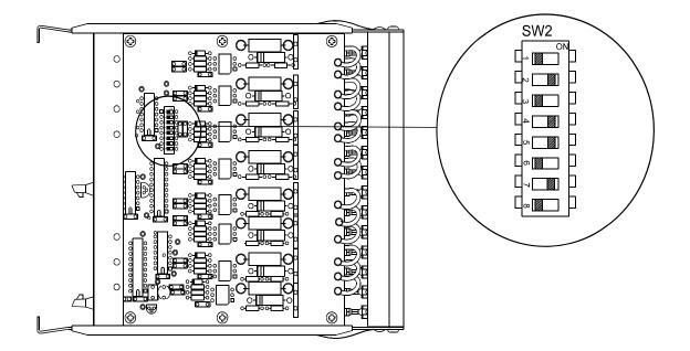
Note: Switch SW2 controls 8 status inputs. As supplied, all switches are in the left hand position and all status inputs are high speed devices. For high stability use, the relevant switch should be moved to
